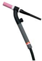
PTA-17, PTA-17V, PTA-17F and PTA-17FV Air-cooled TIG torch, rated 150 amps at 60% duty cycle. The PTA-17V is equipped with a valve for gas flow control. The PTA-17F is equipped with a flexible head for easy maneuverability into tight spaces. The PTA-17FV is equipped with both a gas valve and a flexible head.
